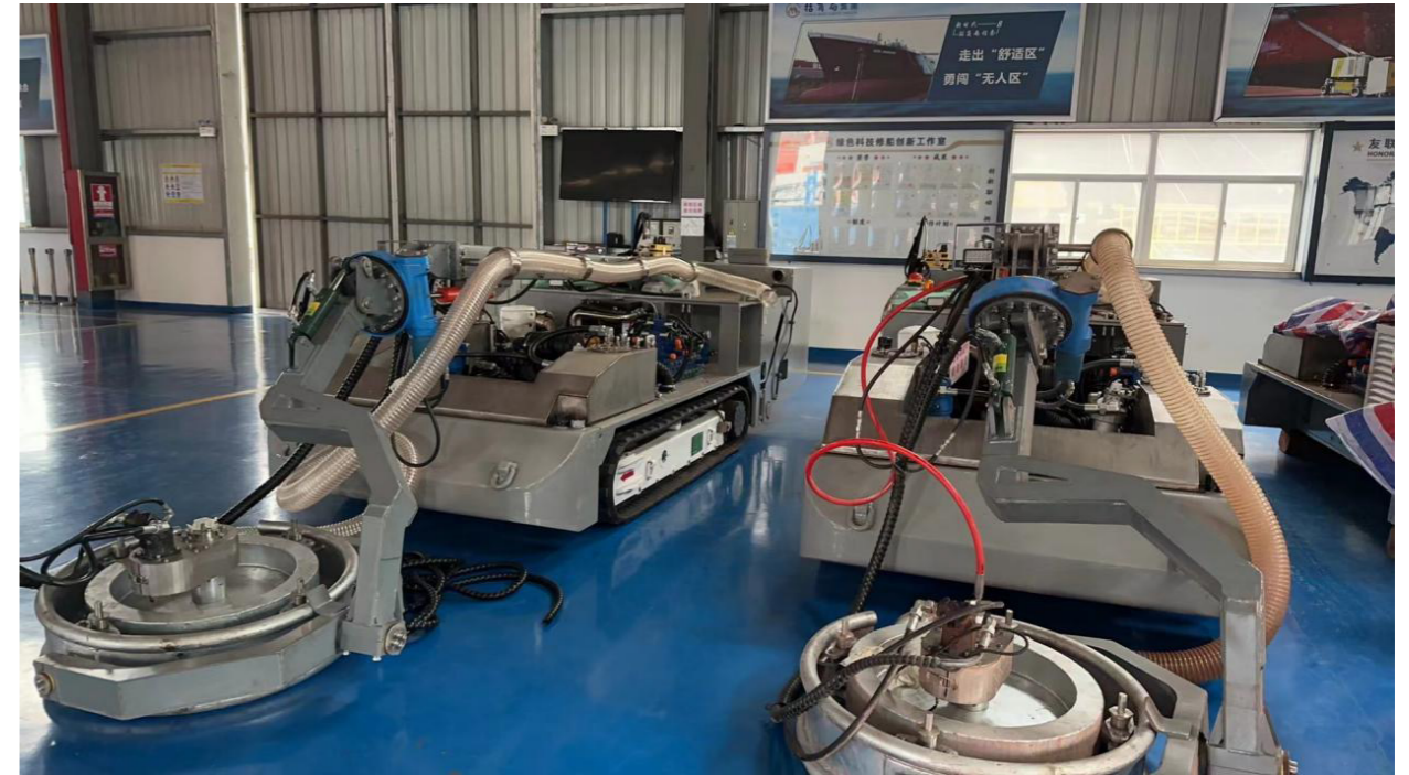
Hyper-pressure Water Blasting Rust Removal
